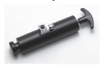
For use with: Fluke 700 Series Pressure Modules and the Fluke 710 Series Pressure Calibrators. **Description:** The Fluke 700PMP is a hand-operated pressure pump to provide pressures up to 150 psi/1000 kPa. Output fitting is 1/8 FNPT.
