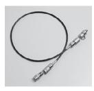
**Description:** The Fluke 700HTH hydraulic test hose is a 10,000 psi, 700 bar working pressure test hose that features stainless steel and nylon construction. The hose uses self-sealing fittings with easy finger tight connections. The hose has very low volumetric expansion and a negligible pressure drop at rated pressures.
