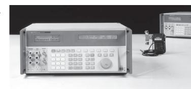
Note: With a Fluke 700PCK and any Fluke Pressure Module, a Fluke 5520A Calibrator becomes a precision pressure standard.
